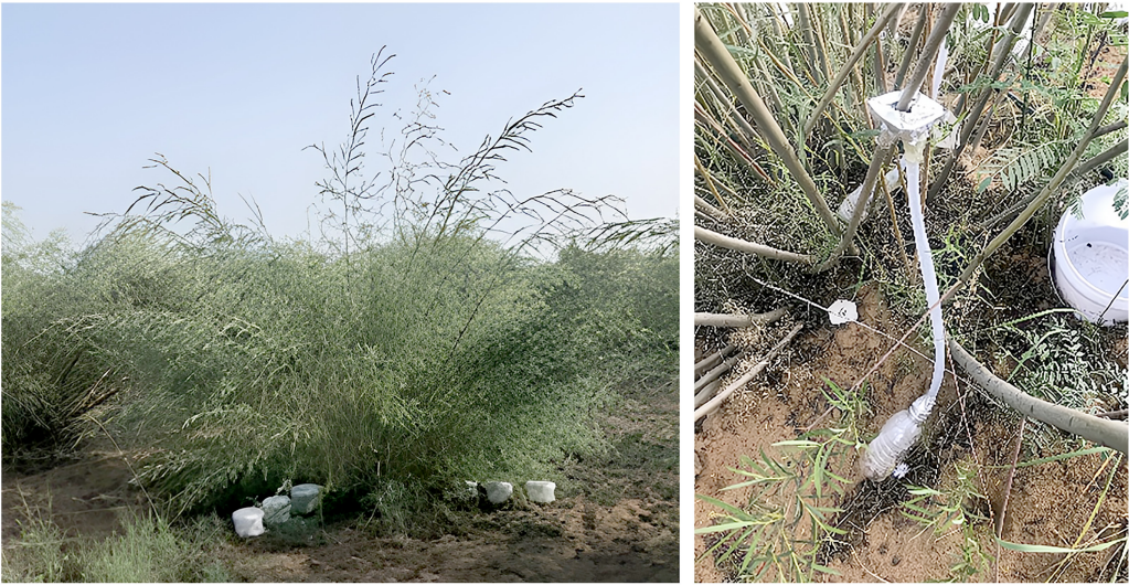
图 2 穿透雨与树干茎流设备布置图 Fig.2 Arrangement of throughfall and stemflow equipment
