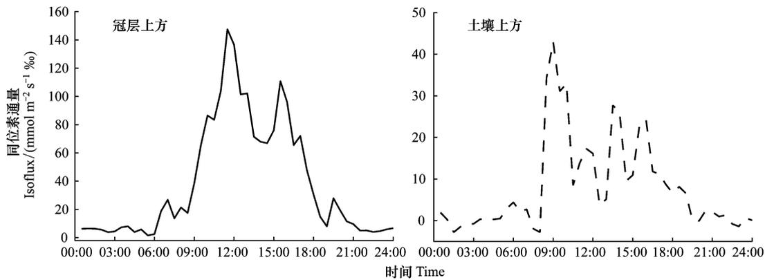
图6 森林冠层上方和土壤上方  $\text{H}_2^{18}\text{O}$  同位素通量的日组分特征Fig.6 Diurnal composites of  $\text{H}_2^{18}\text{O}$  isoflux above the forest canopy (top panel) and near the soil surface (bottom panel)
